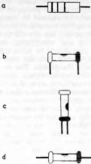
Fig. 2. The four types of resistor found in miniature receivers.
