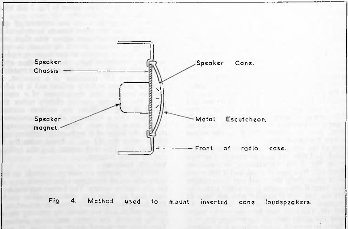
Fig. 4. Method used to mount inverted cone loudspeakers.
