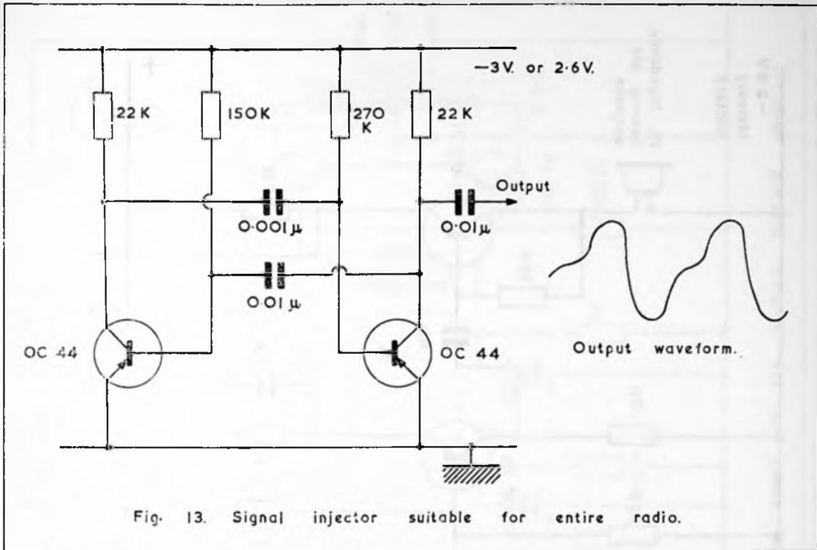
Fig. 13. Signal injector suitable for entire radio.
