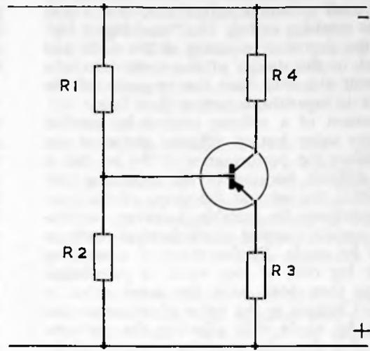
Fig. 3. Transistor bias resistors.
