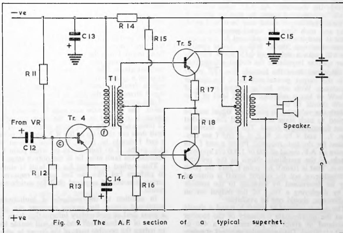
Fig. 9. The A.F. section of a typical superhet.
