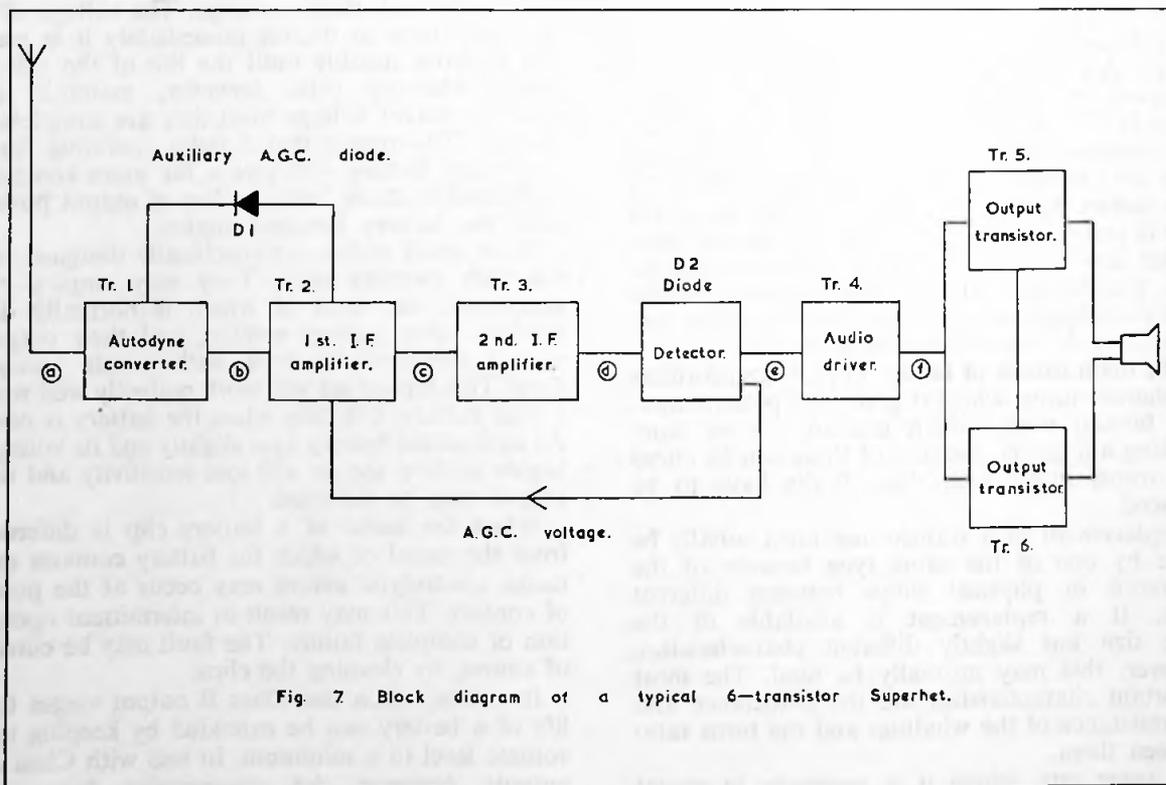
Fig. 7 Block diagram of a typical 6-transistor Superhet.
