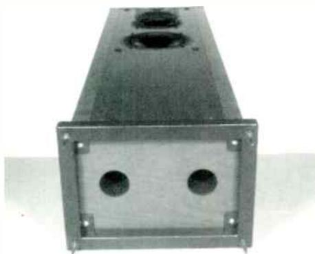
The ports set into the base of Heybrook's Sextet IIs can only operate properly when the 'speakers are raised off the floor on their dedicated spiked stands.
