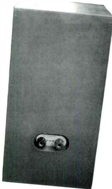
Distinguishing the MkI from the MkII are the former's binding posts. The MkII used an RCA phono connector instead. Other differences in the later model include ceramic magnets instead of alnicos and a wooden front baffle in the place of the MkI's very rigid metal one.
