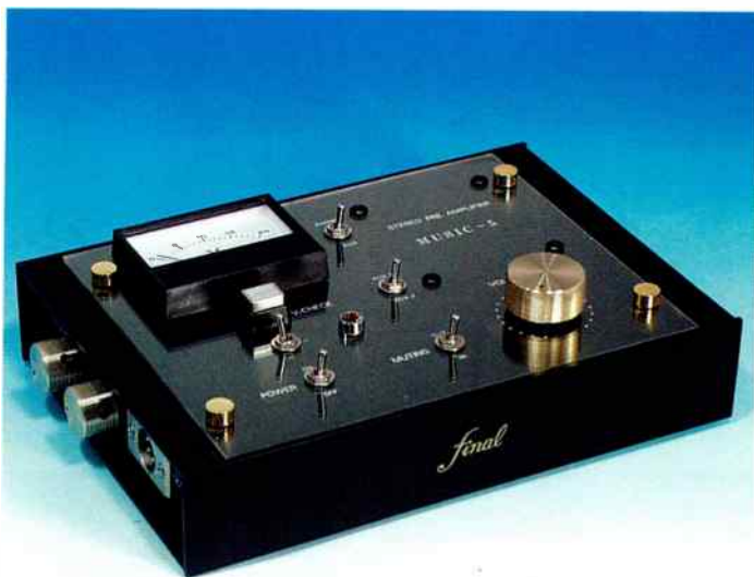
Both the pre and power are housed in classy aluminium extrusions with perspex top plates.
