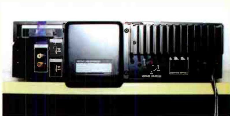
Many better-built older players (like the Pioneer PD-91) had chunky transformers on their hack panels.
