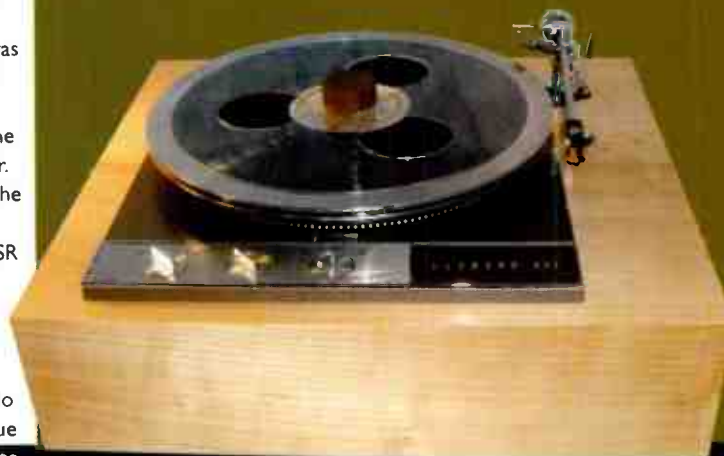
Second stage: drop the record stabilizing ring on the edge of the record and you can now take off the cantering device.
