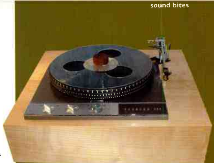
First stage: place cantering device on top of the record.
