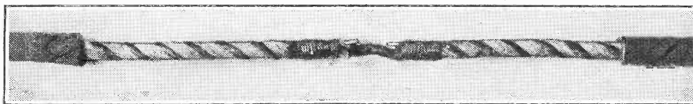
Part-sectioned length of the aerial wire, showing the twisted and overlapping conductors with one of the "breaks," which occur at 1\frac{1}{4} in. intervals.
