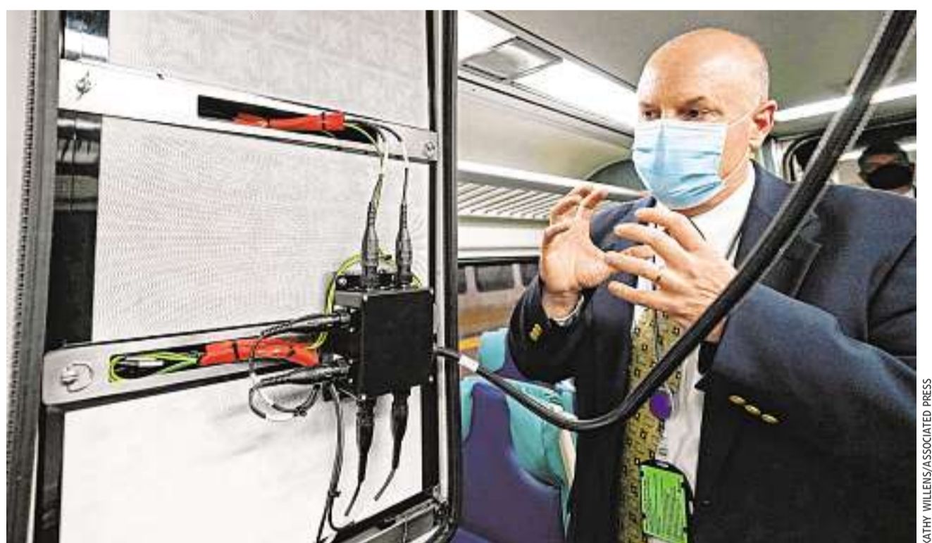
Metro-North Chief Mechanical Officer James Heimbuecher described a test of an air filtration and purification system on a railcar in October.
