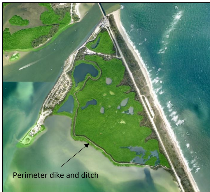
Figure 9. Aerial imagery and land cover of Sebastian Inlet State Park in Indian River County, FL, illustrating wetland alteration by mosquito impoundments. Mangrove (green) and salt marsh (blue) habitats are impounded by a perimeter dike that cuts these areas off from the estuary. Dikes alter normal tidal flow and facilitate invasion by non-native vegetation (Brockmeyer et al. 1996). Land cover data from Florida Cooperative Land Cover version 3.5 (FFWCC/FNAI 2021).
