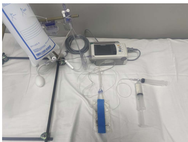
FIGURE 1. The setup used for measuring pressure includes a Philips IntelliVue X2 patient monitor, an arterial line transducer setup connected to a 100-mL saline bag, protective strip on the saline bag, and 2 syringes filled with saline connected to the saline bag with a stopcock to allow for creating a closed system after the initial column of saline is added.
