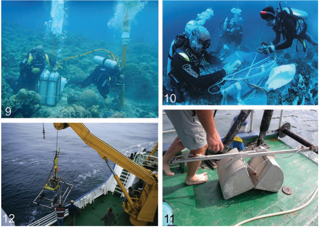
Figs 9–12: 9, airlift sampler, Panglao, Philippines (photo: Panglao 2004 Marine Biodiversity Project); 10, brushing, Panglao, Philippines (photo: Panglao 2004 Marine Biodiversity Project); 11, Van Veen grab, Rovinj; 12, Reineck box sampler on R/V Senckenberg.
