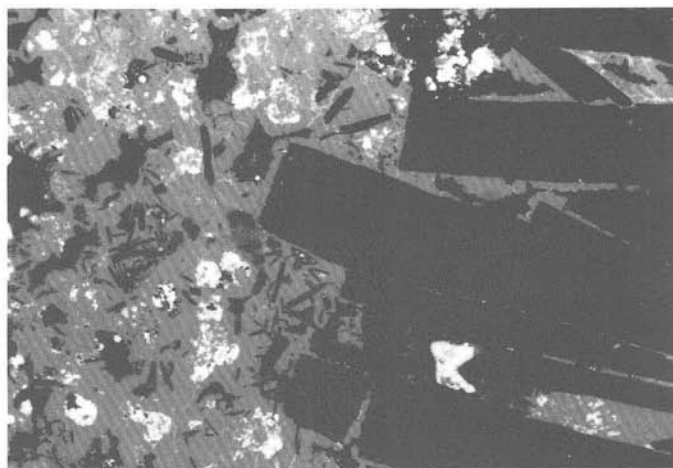
Fig. 10. Sample SO 41-181 FG 6. Schalenblende (medium gray) encloses fine-grained, occasionally spheroidal pyrite (light gray, almost white), galena (light gray) locally in delicate, rhythmic to concentrically layered alternations, and numerous small euhedral plates and crystal aggregates of barite (dark gray, almost black). At times galena, partly associated with covellite (dark gray), constitutes fine-grained interstitial fillings and cements narrow fractures and/or shrinkage cracks in schalenblende. The latter occupies interstices within the adjacent coarse crystal aggregate of barite and coats, partly as a thin “intergranular film”, its large plates euhedrally developed after {001}. At one place schalenblende heals a fracture, while it is in turn thinly coated by galena. Gangue material, natural cavities and pores (all likewise dark gray, almost black). Polished section, \times 65 .
