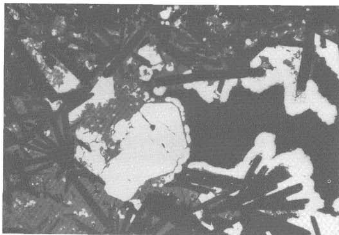
Fig. 17. Sample SO 41 -181 FG 9. Schalenblende (dark gray) comprises abundant inclusions of barite crystal aggregates (black) along with small amounts of galena (light gray) and pyrite (light gray, almost white), which locally forms spheroids. Schalenblende completely fills the interstices within crystal aggregates of barite. Overgrowth of galena produced a larger euhedral aggregate which is peripherally, very thinly in places, coated by schalenblende, which is itself in turn rimmed by pyrite (light gray, almost white). The latter also exhibits rims around euhedral barite plates or their thin schalenblende coatings ("films") and furthermore occupies interstices among the barite crystal aggregates. Natural cavities and pores (both likewise black). Polished section, oil immersion, \times 65 .
