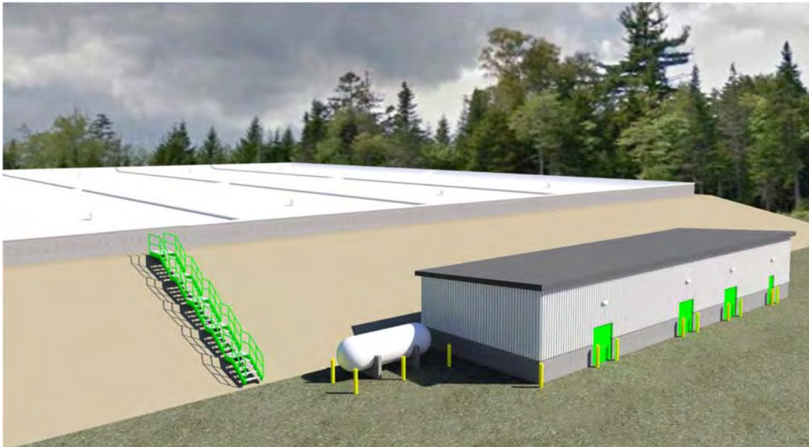
Figure 14. Three-dimensional model showing the pump house of the low-rate anaerobic digester proposed for the Lake Utopia Paper Mill in Utopia, New Brunswick.
