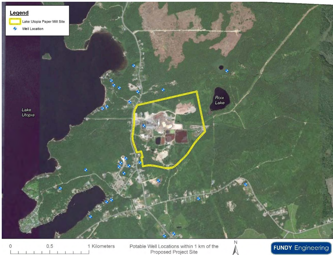
Figure 32. Aerial photograph showing groundwater wells on file with the NBDELG within a 1 km radius around PID 15079221, which is part of the Lake Utopia Paper Mill in Utopia, New Brunswick. The well logs and water quality records were obtained for characterizing local groundwater quantity and quality.
