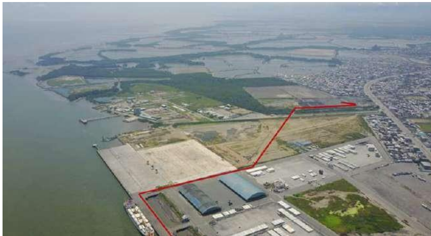
Figure 53: Sediment Dredging Piping SEDIMENT DREDGING PIPING ROUTE
