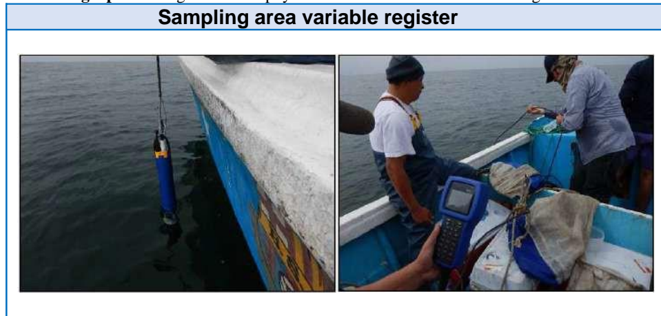
Photograph 36: Registration of physicochemical variables with YSI signature EXO2 CTD
