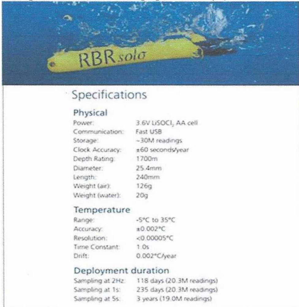
Figure No. IV-5: RBR Solo tide gauge Technical Specifications
