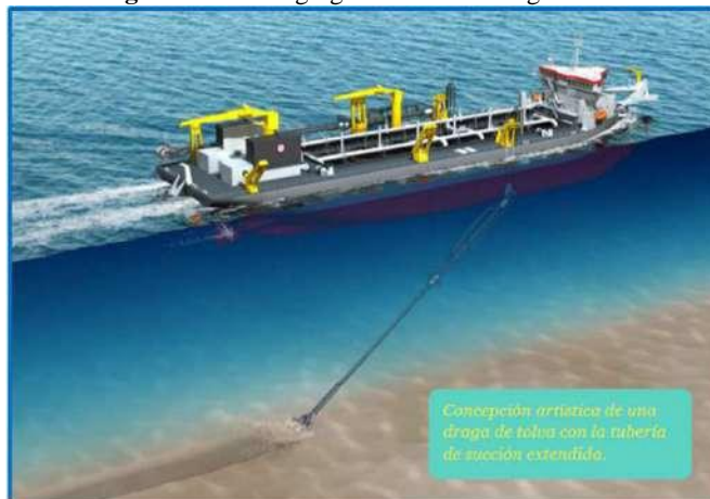
Figure 227: Dredging mechanics Dredge TSHD
