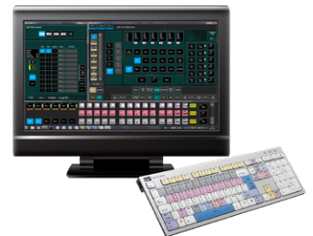
KSP Control Surface provides a software and keyboard option for operating K-Frame.
